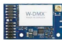
The transceiver supports our innovative Flex mode, meaning the card can be quickly and easily changed between transmitter and receiver.
