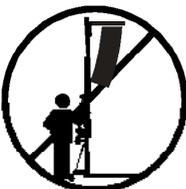
**3.8** - NEVER move the lift whilst it is carrying a load. It is not advisable to carry out any type of horizontal movement even small positional adjustments.
