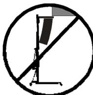
**3.10** - Take care with all obstacles above the lift and its extension zone such as cornices, balconies, and luminous signboards. It is very important to avoid the presence of all types of cables below the extended lift.
