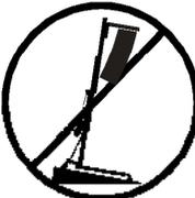
**3.2** - Only place the lift on hard, flat surfaces always checking that it is in a vertical position by using the bubble level indicator (**L**) found on the base. Adjust the leg stabilizers (**Q**) by turning the handles (**H**) to level if necessary. NEVER use wedges or other foreign objects to balance the lift.
