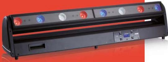
All the amazing features and performance of the award winning Robe LEDWash luminaires in a 1000 mm moving linear strip. 8 individually controlled 15W RGBW LED modules equally spaced along the strip with fully adjustable zoom from 12–67 degrees. The strip itself has a very fast 270 degree tilt movement which can be precision indexed or programmed to produce rapid sweeping movements.
