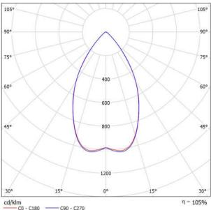
Luminaire classification according to CIE: 100 CIE flux code: 89 99 100 100 105
