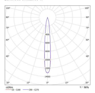
Luminaire classification according to CIE: 100 CIE flux code: 98 100 100 100 98
