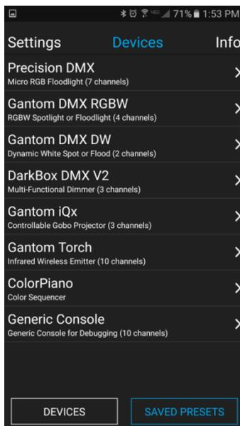
First, open the **DMX Programmer** app by Gantom. The app will open to the screen you see here. From this screen, select either the Gantom DMX RGBW or the Gantom DMX DW.
