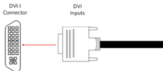
An HDMI input is connected to the DVI-I connector using a DVI-HDMI Adaptor:
