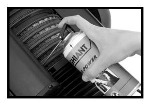
To clean the shutters: Use dry air to clean and a vacuum cleaner to remove dust and other loose particles.
