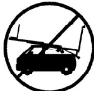
3.13 - All sections must be lowered first, and the legs placed in its transport position, before transportation.
