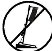
**3.2** - Only place the lift on hard, flat surfaces always checking that it is in a vertical position by using the bubble level indicator (**L**) found on the base section. Adjust the leg stabilizers (**Q**) by turning the handles (**H**) to level if necessary. NEVER use wedges or other foreign objects to balance the lift.
