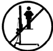
**3.1** - The TE-071 is a machine designed to elevate loads upwards in a vertical direction, It should NEVER be used as a platform to elevate people.
