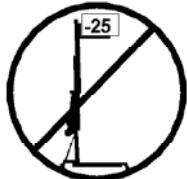
3.15 - The minimum load to avoid problems regarding the braking mechanism is 25Kg. Without this load the brake will not work.
