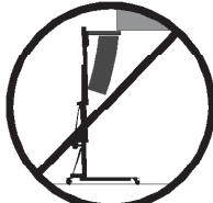
**3.10** - Take care with all obstacles above the lift and its extension zone such as cornices, balconies, and luminous signboards. It is very important to avoid the presence of all types of cables below the extended lift.
