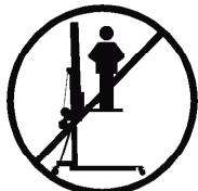
**3.1** - The TL-A150 is a machine designed to elevate loads upwards in a vertical direction. It should NEVER be used as a platform to elevate people.
