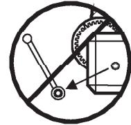
**3.16** - NEVER take apart the crank of the winch when the lift is carrying a load or extended.
