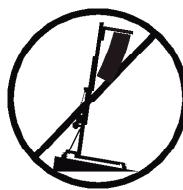
**3.2** - Only place the lift on hard, flat surfaces always checking that it is in a vertical position by using the bubble level indicator (**L**) found on the base. Adjust the leg stabilizers (**Q**) by turning the handles (**H**) to level if necessary. NEVER use wedges or other foreign objects to balance the lift.
