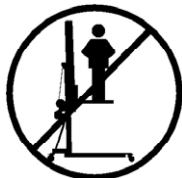
**3.1** - The TE-086 is a machine designed to elevate loads upwards in a vertical direction, It should NEVER be used as a platform to elevate people.
