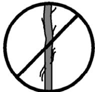
3.12 - Before using the lift, check the condition of the cable. The cable should not have broken threads or show any signs of crushed/flattened areas. NEVER use faulty cables, always change them if there is any doubt. Only use VMB steel cables; reference: DIN 3060. Quality: 180KG/mm and torsion resistant.
