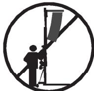
**3.8** - NEVER move the lift whilst it is carrying a load. It is not advisable to carry out any type of horizontal movement even small positional adjustments.
