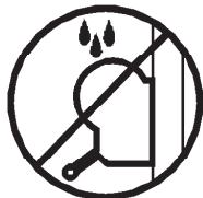
**3.14** - Do not grease or lubricate the winch's braking mechanism. The brake disks have been greased with a special heat and pressure resistant solution. Other products should not be used to avoid negative effects regarding the braking mechanism.
