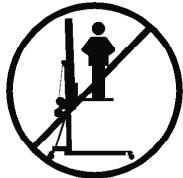
**3.1** - The TE-076 is a machine designed to elevate loads upwards in a vertical direction. It should NEVER be used as a platform to elevate people.
