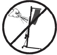
**3.7** - If there is a possibility of strong winds or gusts, place the lift on the ground firmly and secure it with the use of straps. NEVER attach a strap to a vehicle or any other object that can possibly be moved.
