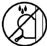
3.14 - Do not grease or lubricate the winch's braking mechanism. The brake disks have been greased with a special heat and pressure resistant solution. Other products should not be used to avoid negative effects regarding the braking mechanism.
