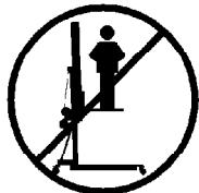
**3.1** - The TE-046 is a machine designed to elevate loads upwards in a vertical direction, It should NEVER be used as a platform to elevate people.
