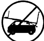
3.13 - All sections must be lowered first, and the support system (**SA**) must be locked with the catch pawl (**R**), before transportation.
