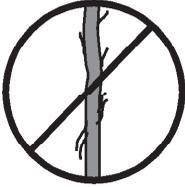
**3.12** - Before using the lift, check the condition of the cable. The cable should not have broken threads or show any signs of crushed/flattened areas. NEVER use faulty cables, always change them if there is any doubt. Only use VMB steel cables; reference: DIN 3060. Quality: 180KG/mm and torsion resistant.
