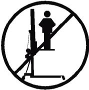
**3.1** - The TE-034 is a machine designed to elevate loads upwards in a vertical direction, It should NEVER be used as a platform to elevate people.
