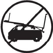
**3.13** - All sections must be lowered first, and the support system (**SA**) must be locked with the catch pawl (**R**), before transportation.
